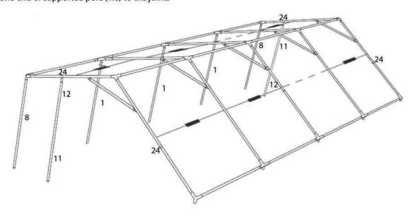
Attach the another supported poles (1.8) to the joints, built-up the framework.
