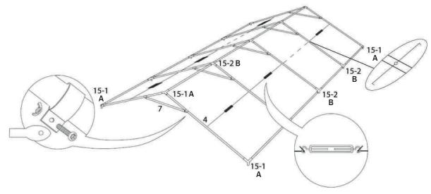
Attach one end of supported pole (1.8) to the joints
